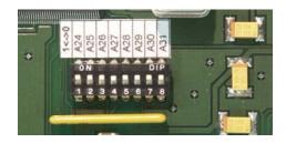
This Standard/Extended address range switch is marked on the print with "S/E". Standard address range (A24) is selected with the switch in the Down-position. The extended address selector switch (A31..A24) is then disabled.
