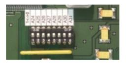
This Standard/Extended address range switch is marked on the print with "S/E". Standard address range (A24) is selected with the switch in the Down-position. The extended address selector switch (A31..A24) is then disabled.
